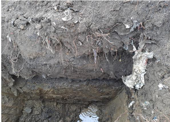
**Fig 6C** At TP22, Topsoil overlies a dark brown to brown sandy gravelly CLAY with rare plastic and cobble-sized concrete blocks. Possible Made Ground continues to 1.50m with an organic signature. This is thought to be buried topsoil / subsoil.
