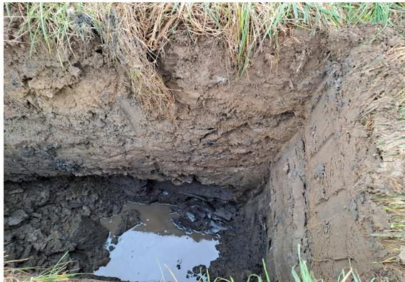
**Fig 7B** At TP07, topsoil was found overlying a firm brown slightly sandy slightly gravelly SILT/CLAY with rare anthropogenic content. Stiff grey sandy gravelly silty CLAY persisted from 1.10m to 1.80m. From 1.80m to the pit base at 2.50m, possible highly weathered rock was recovered as clayey/silty GRAVEL. Again, as with TP05, a moderate water strike was recorded towards the base of the pit at 2.30m.
