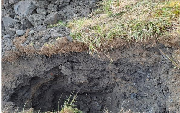
**Fig 6B** At TP13, >2% plastic / rubbish was recorded in the Clay Made Ground to a depth of 1.40m (56.02m OD).
