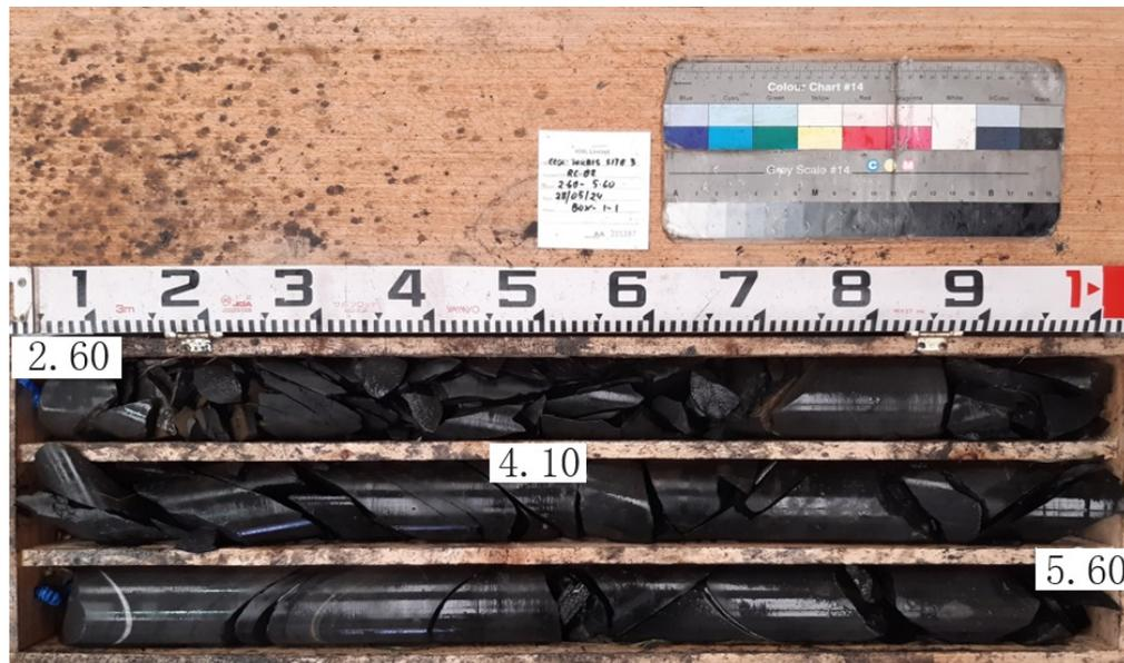
Discontinuity spacings in the rotary cores generally ranged from medium (200 to 600mm) to closely spaced (60 to 200mm), rarely widely (600 to 2000mm) spaced. The discontinuity surfaces were typically smooth to locally rough, planar to locally curvilinear. Apertures were tight to locally partly open with local clay smearing. Discontinuities host calcite veinfill (from 1-20mm thick). Dips are subhorizontal, 10° to 15°, rarely 40° to 45° and very locally 70°.
